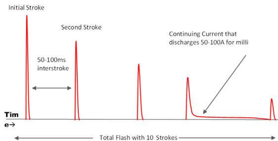
Since the peak current seldom exceeds a few 10s of kA, it does not have the same effect on the arresters as a high current stroke. The charge carried by the stroke can easily exceed 10coulombs (IEEE 1410). With this stroke charge, the standard heavy duty arrester is immediately pushed beyond its 1 coulomb thermal rating. Although never recorded in the field, it is only logical that this failure mode occurs almost as often as multi-stroke lightning does. .
